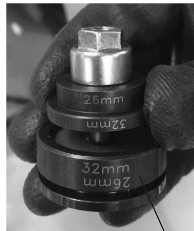
1 upper cutting disc with two diameters:
